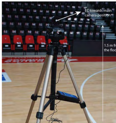
Main camera illuminance (EC) measurement
